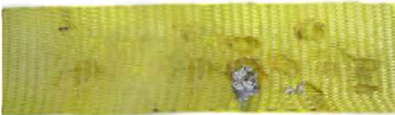
WELDING SPARK DAMAGE
